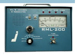
An excellent ratemeter for labs and frisking stations. This is an all-digital instrument with a preferred analog display that automatically chooses the correct range with no user intervention required. Powered by line or battery for up to 24 hours. Relay outputs enable the use of external lights, sirens, etc.
